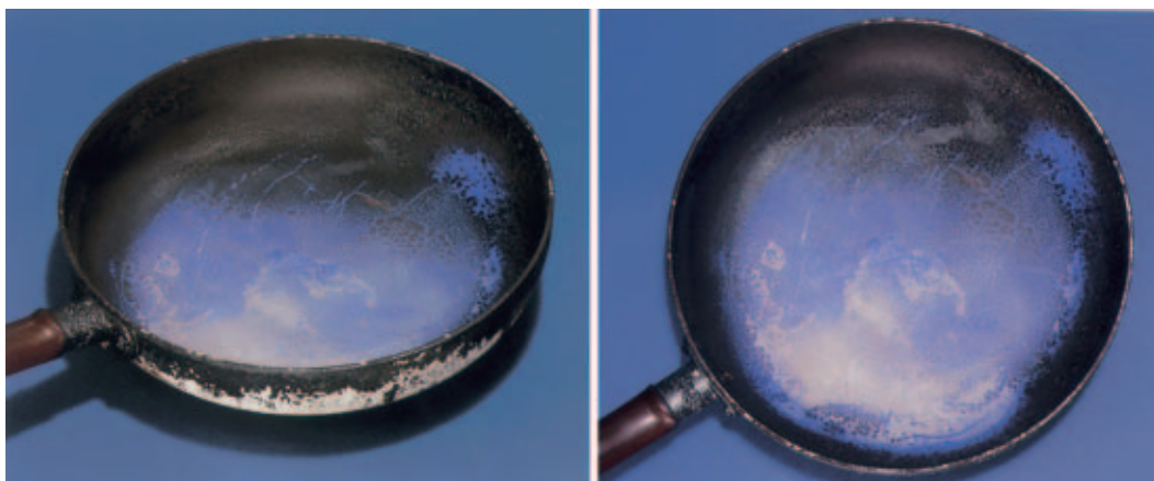
Fig. 3 The frying pan coated with PTFE. The Teflon ® that had coated the bottom of the pan came off, and the iron thus exposed appeared blue-white.
